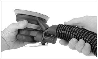
**Figure 3.** Attaching sander to 11/4" canister vacuum hose.
